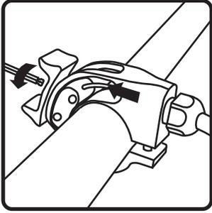
**7a.** Loosen set screw in lever. Feed cable from shock collet to lever and tighten lever set screw securing cable.
