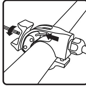
**7b.** Loosen set screw in lever. Feed cable from shock collet to lever and tighten lever set screw.
