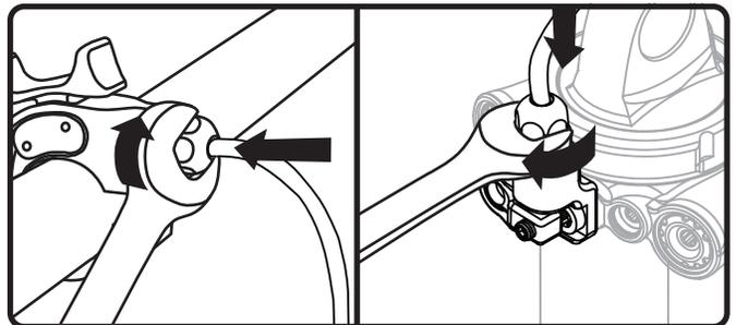
**4.** Using the retained set screw install the shock side actuation lever and collet.
