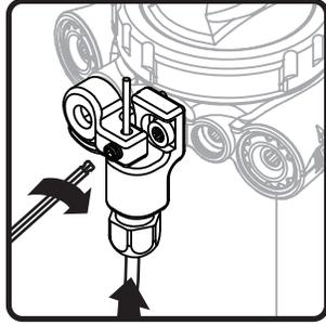
**8a.** Place CS lever in on position and tighten set screw. Trim cable as short as possible and cap end.
