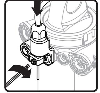
**8b.** Place CS lever in on position and tighten set screw. Trim cable as short as possible and cap end.
