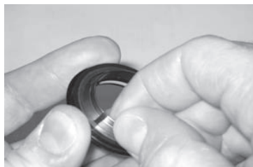
Fig.1 - Use one hand to push one side of split in compression ring towards center.
